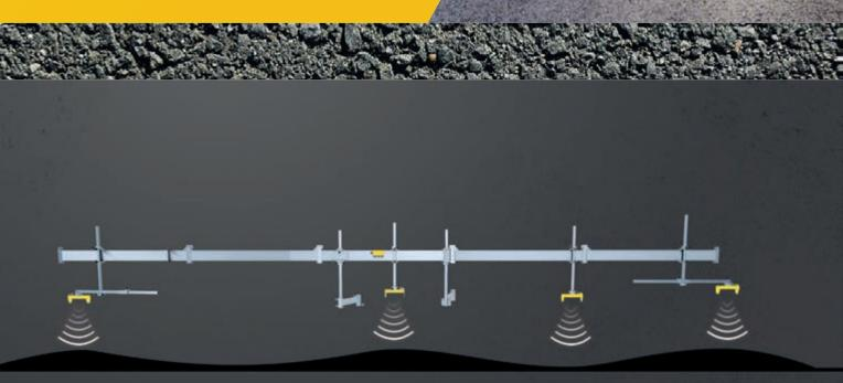
As a combination, **MOBA-matic** and the sensor solution **Big Sonic-Ski** with up to 4 ultrasonic sensors are absolutely unbeatable! Thanks to a span of up to 13 m, even long ground waves are completely levelled out and eliminated. This unique feature ensures an exceptionally flat surface and makes the system not only the most precise technology on the market, but also an absolutely groundbreaking solution. Welcome to road construction of the future!
